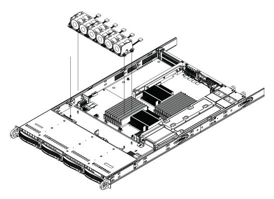
Figure 6-2. System Cooling Fans
